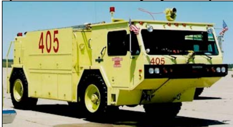
Figure 32 - Typical MCAS P-19 ARFF Vehicle
